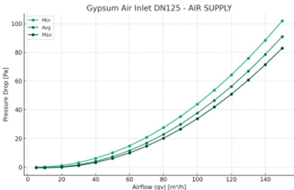
The chart presented here shows pressure drops with "Min", "Avg", and "Max" values, in relation to the airflow (qv) through the gypsum air inlet DN125 ("Gypsum Air Inlet DN125 - AIR SUPPLY"). The lines reflect different levels of pressure drops at various airflow volumes.
