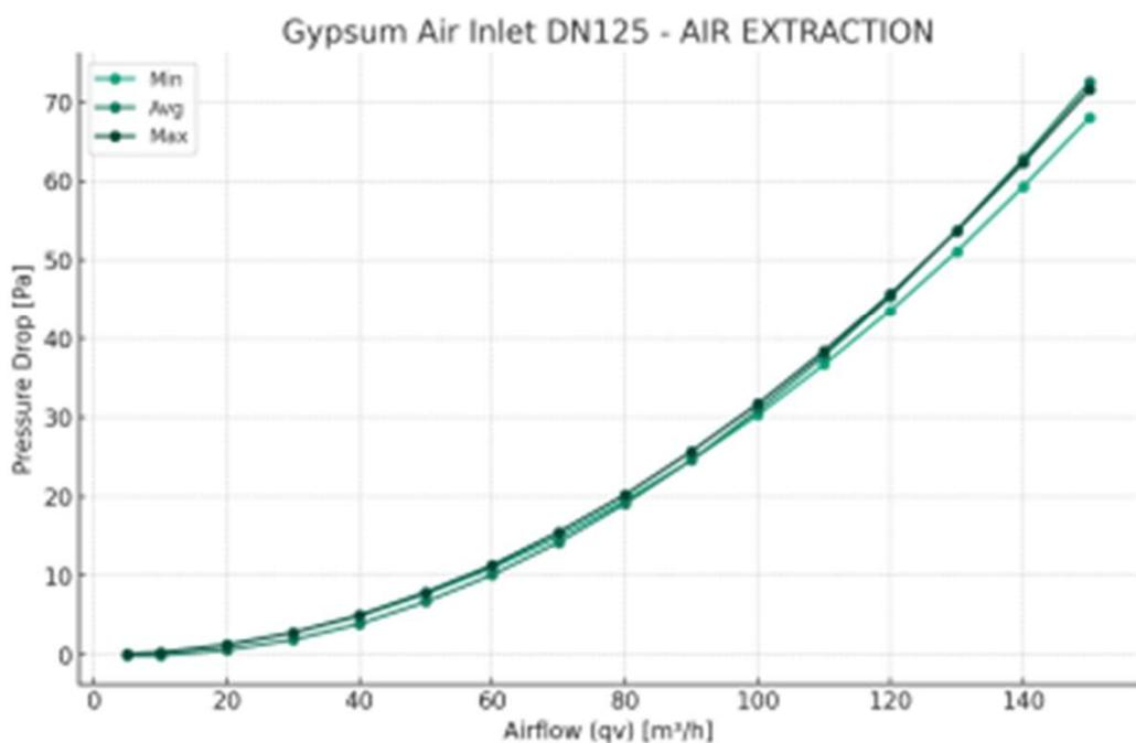
Here is the visualization for the Gypsum Air Inlet DN125 - AIR EXTRACTION, displaying the pressure drop (Pa) against the airflow (qv in m³/h) with "Min", "Avg", and "Max" values
